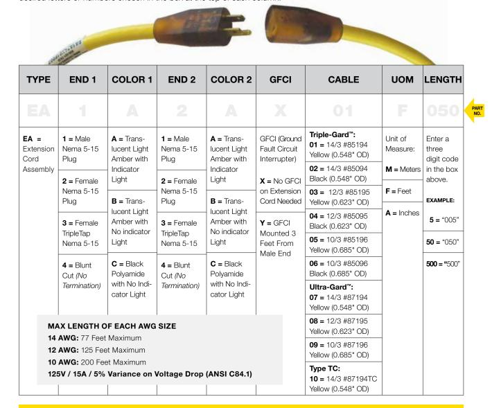
In the sample part number above, **EA1A2AX01F050** is a double ended extension cord assembly using 14/3 Yellow Triple-Gard™ Portable Cord (#85194) and is 50 feet long. End 1 is a Male Nema 5-15 Plug and End 2 is a Female Nema 5-15 Plug, both are a translucent light amber color with an indicator light.
