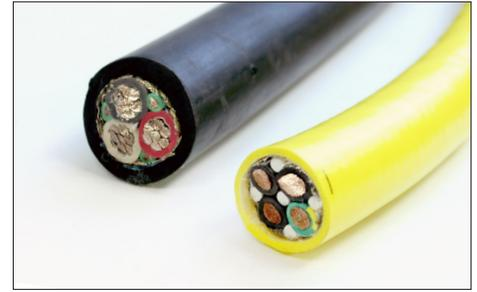
Motor size will dictate the preferred cable configuration. For larger sized motors, cables using 3 symmetrical grounds are preferred to minimize induced voltages into the ground circuit. For smaller motors, 4-conductor cable designs are sufficient.
