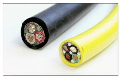
Motor size will dictate the preferred cable configuration. For larger sized motors, cables using 3 symmetrical grounds are preferred to minimize induced voltages into the ground circuit. For smaller motors, 4-conductor cable designs are sufficient.
