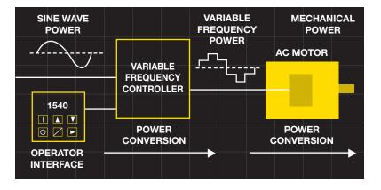
Typically, the AC output of the VFD from the IGBTs is a PWM (Pulse-Width-Modulation) signal. The PWM output generates a series of pulses of varying width (or frequency). By varying the width of the pulses, the average power generated resembles a sine-wave output. It is important to note, discussed later in this paper, the switching speeds of the IGBTs typically operate in the 10-20 kilohertz range.
