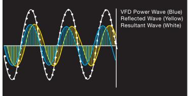
The Resultant Wave (White) is a combination of the VFD Power Wave (Blue) and the Reflected Wave (Yellow). The Resultant Wave amplitude is the sum of the Power Wave and the Reflected Wave amplitudes. When the VFD Power Wave and Reflected Wave peaks are in alignment, the Resultant Wave amplitude can be as much as 2X the "original" Power Wave.
