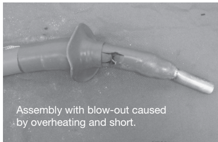
Actual failure determined to have been caused by damage to insulation during installation of the termination kit.
