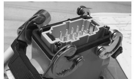
Notice the coding pins that can be used to prevent installation errors
